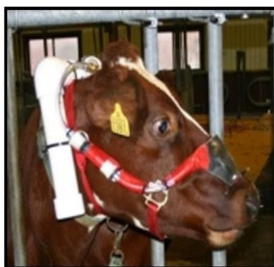
After the sampling collection period has been completed, the canister taken off the animal and connected to the dilution system and the final pressure recorded. Nitrogen is then slowly added until the pressure in the canister is increased to about 1.2 ATM. Another pressure
