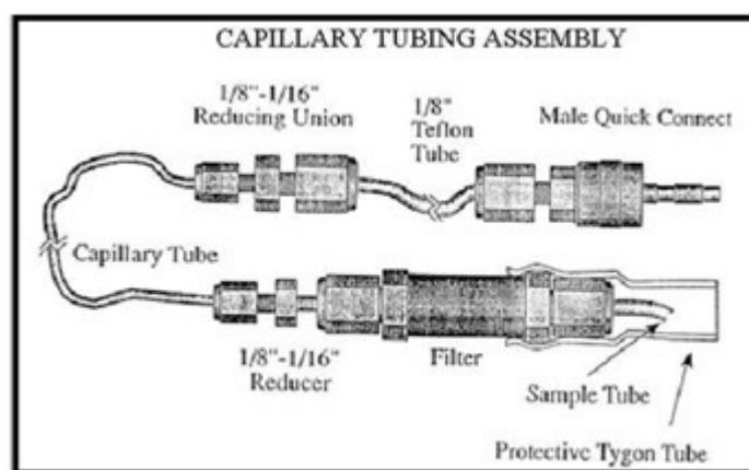
The length of the capillary tubing regulates the sampling rate. Stainless steel capillary tubing with an inside diameter of .005" and an outside diameter of 1/16" serves as the flow restrictor and transfer line. Short sample integration periods (e.g. 1 hr) may require only a short piece of tubing while longer periods (e.g. 24 hr) require much longer lengths of tubing.
