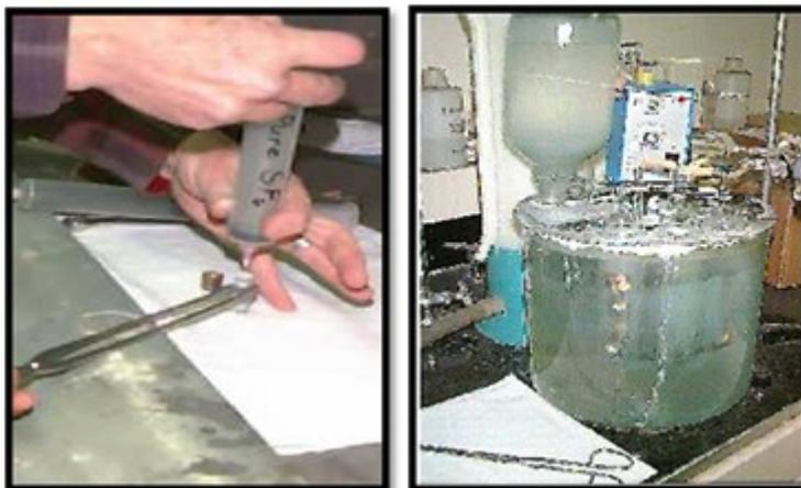
The tube should then be placed in a glass receptacle, in a 39°C water bath. A small flow of clean N<sub>2</sub> gas is maintained to purge the glass receptacle of SF<sub>6</sub> emissions. Weights of each tube should be taken weekly to determine the release rate of SF<sub>6</sub>. Five to six weeks is generally required to gain a good idea of the release rate.
