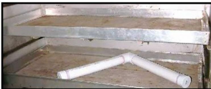
After assembling the PVC pieces, and allowing the glue to dry (12-24hr), place the entire assembly into a 120 – 135°C oven for 5-10min. Keep checking the pipe by squeezing it until
