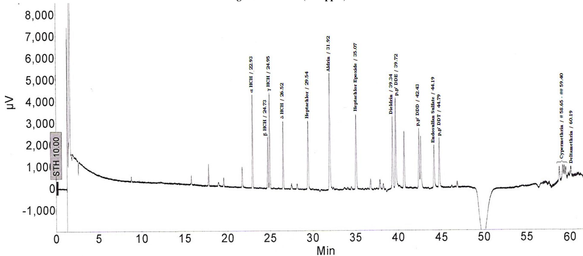
**Fig. 2: Elution pattern and mean retention time of organophosphorous pesticides from standard pesticide mixture using TSD detector (0.01 ppm)**
