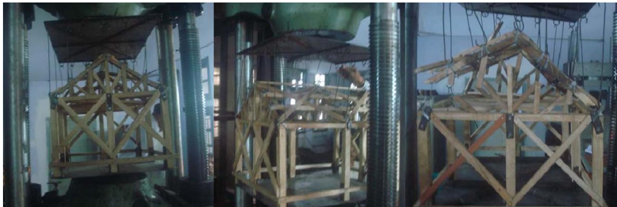
Fig 6: Experimental setup under suction force in UTM
