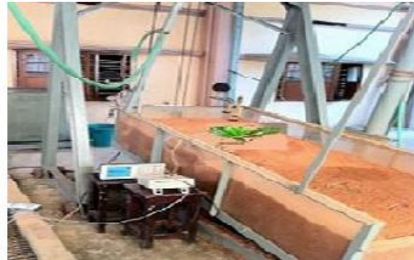
Figure 5. Experimental landslide setup showing the tilt variability
