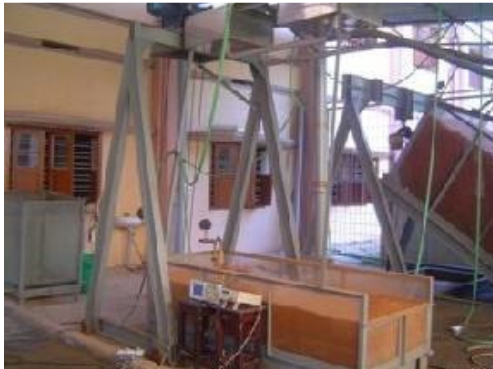
Figure 4. Landslide experimental setups: Left-medium scale, Right-large scale
