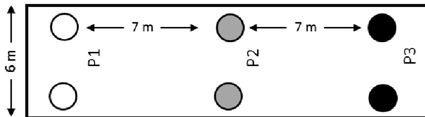
Figure 1. Distribution of the access tubes for field calibration.
