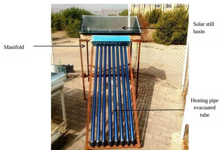
Fig. 8: Heating Pipe Evacuated Tube Solar Still
