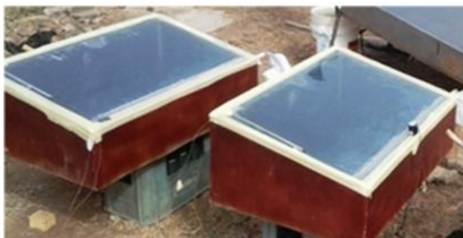
Fig. 4: Solar Still with Submerged Flat Plates
