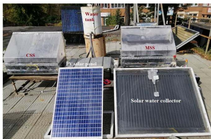
Fig. 11: Modified Solar Still
