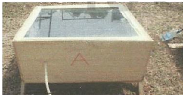
Fig. 3: Single Slope Solar Still with Variable Collector
