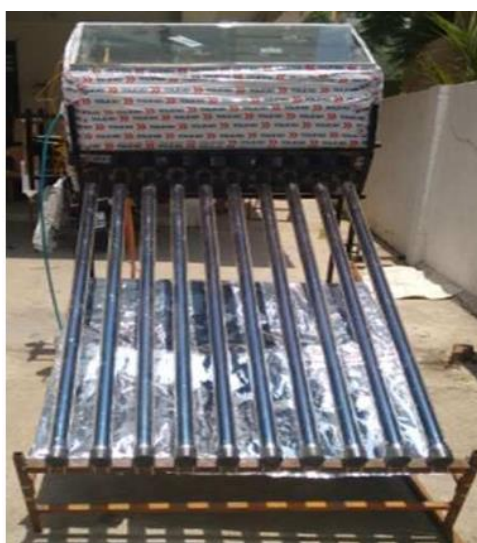
Fig. 5: Double Basin Solar Still Augmented with Evacuated Tubes
