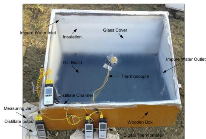
Fig. 7: Single Basin Single Slope Solar Still
