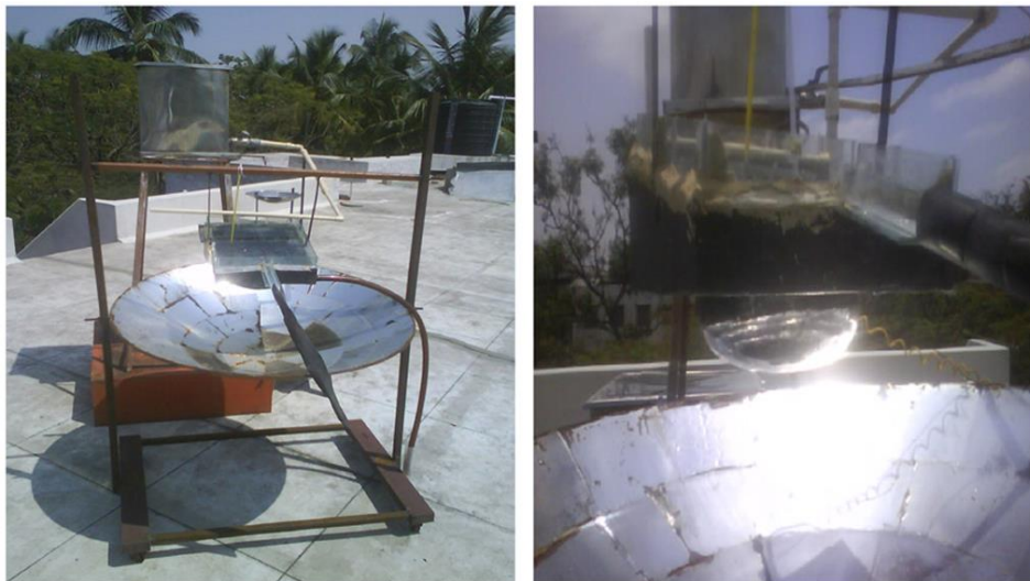
Fig. 1: Concentrator-Coupled Hemispherical Basin Solar Still with Built-In PCM
