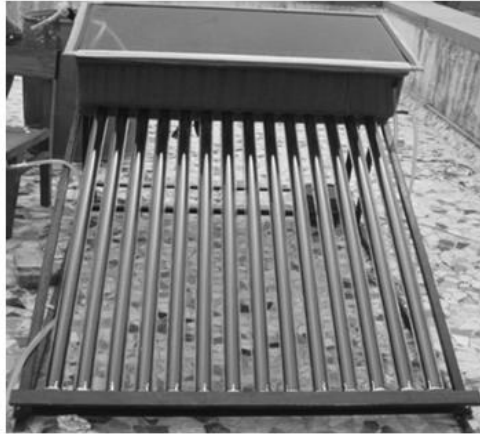
Fig. 2: Pictorial view of double basin solar still with evacuated tubes.
