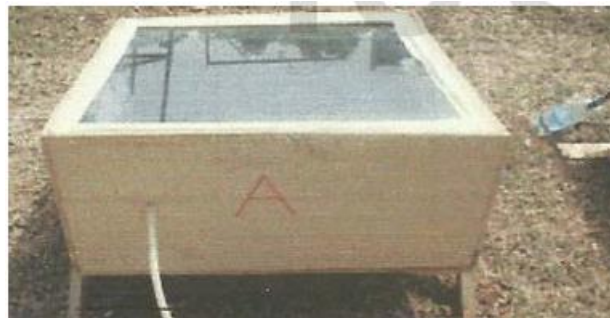
Fig. 3: Single Slope Solar Still with Variable Collector
