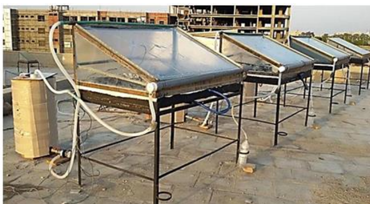
Fig. 6: Solar Stills with Cooling Arrangement for Glass Cover
