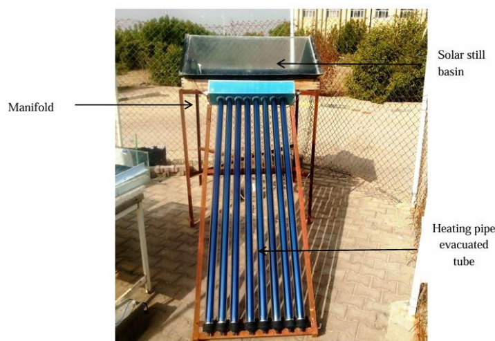
Fig. 8: Heating Pipe Evacuated Tube Solar Still
