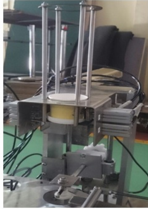
Figure 16: Fourth station (lid placing)
