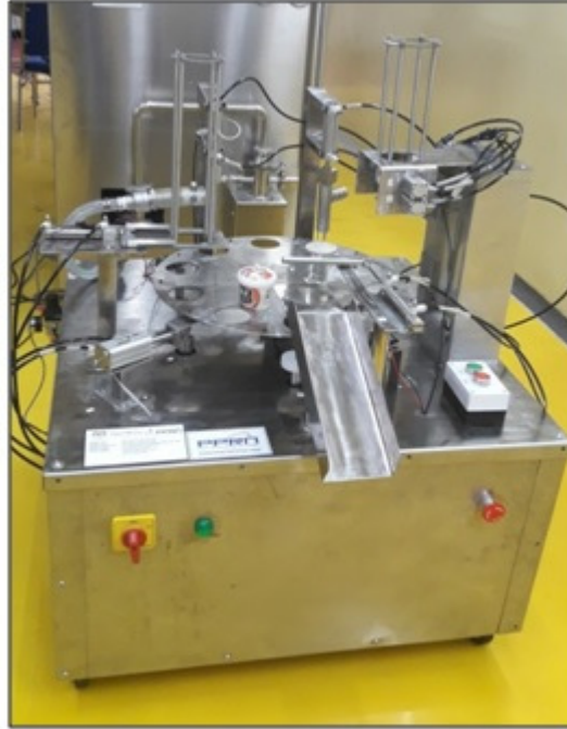
Figure 12: Ice cream filling machine
