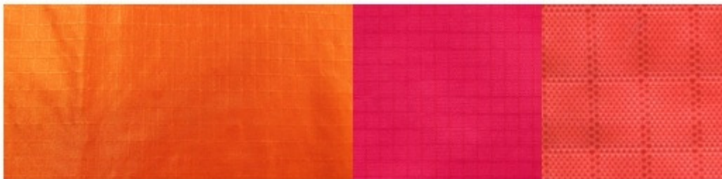
Figure 4. Nylon ripstop fabric for parachutes
