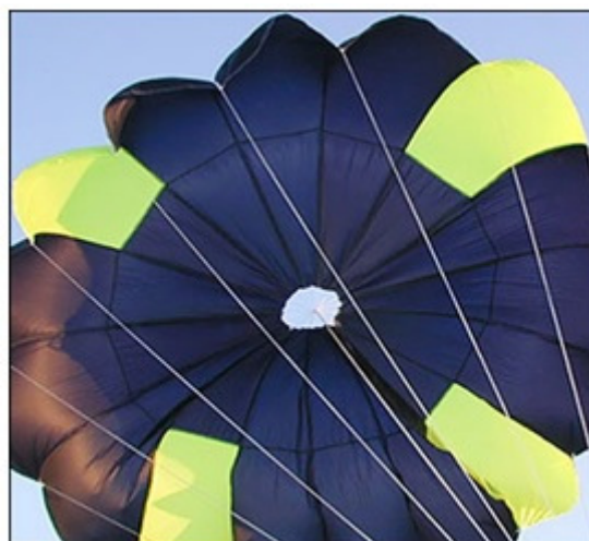
Figure 5. Zero porosity ripstop nylon for canopy cloth
