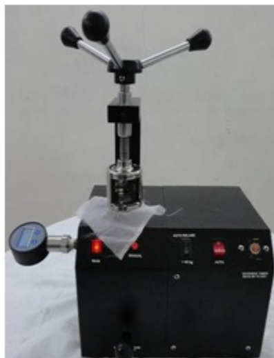
Figure 14. Digital Bursting Strength Tester
