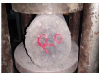
Figure 2.4 Split tensile strength test
