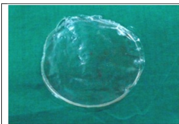
Fig-1: Photograph showing calcium-silver (35:55) nanocomposite films
