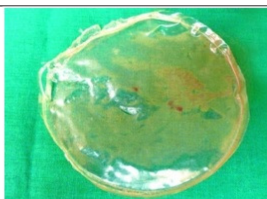
Fig-2: Photograph showing calcium-silver (45:45) nanocomposite film
