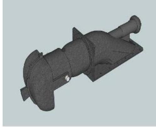
**Fig.6** Shape of water-jet
