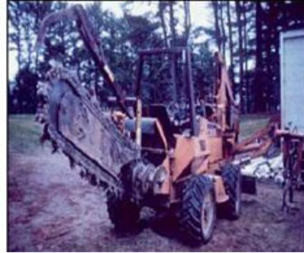
**Fig. 2** Ditchwitch 1260 cutting machine
