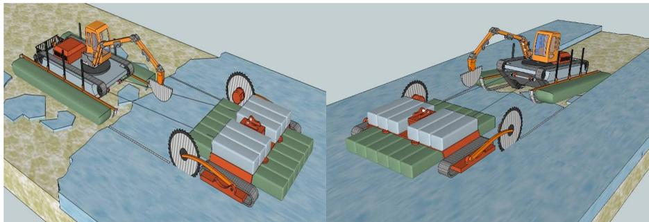
**Fig.13** working process of the amphibious ice-broken vehicle
