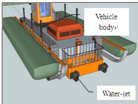
**Fig.7** Installation diagram of slip parts and airbag
