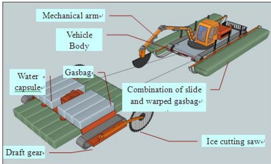
**Fig.4** Main structure of the ice-broken vehicle
